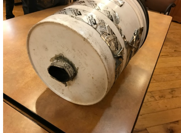
Beevac close up of suction side (left); beevac close up of side connecting to a shop vac (right)
